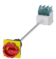
SENTRON, Switch disconnector 3LD, emergency switching-off switch, 3- pole, lu: 25 A, operating power / at AC-23 A 400 V: 9.5 kW, floor mounting with door coupling, rotary operating mechanism, Red / yellow, 4-hole mounting of the handle
