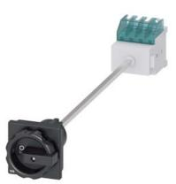
SENTRON, Switch disconnector 3LD, main switch, 4-pole, Iu: 16 A, Operating power / at AC-23 A at 400 V: 7.5 kW, floor mounting with door coupling, rotary operating mechanism, black, 4-hole mounting of the handle
