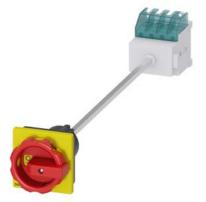
SENTRON, Switch disconnector 3LD, emergency switching-off switch, 3- pole, lu: 16 A, operating power / at AC-23 A 400 V: 7.5 kW, floor mounting with door coupling, rotary operating mechanism, Red / yellow, 4-hole mounting of the handle
